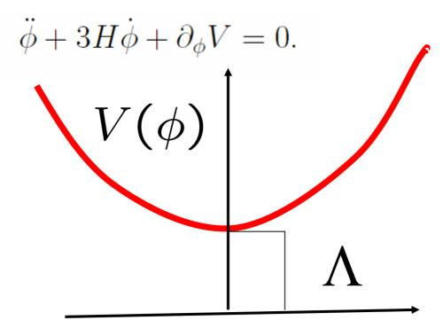
Friction term means system will settle to bottom of potential regardless of initial conditions This is the attractor.
