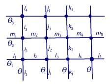
To explain this rather busy picture, the vertical and horizontal lines are labeled by rapidities  $\theta$  or  $\theta_i$ , a line segment is labeled by a basis vector  $i,j,k,\ldots$  of the representation  $\rho$ , and a crossing is labeled by the appropriate R-matrix. The problem of statistical mechanics is to compute the "partition function" by summing over labels, with each set of labels being weighted by the product of the appropriate R-matrix elements.
